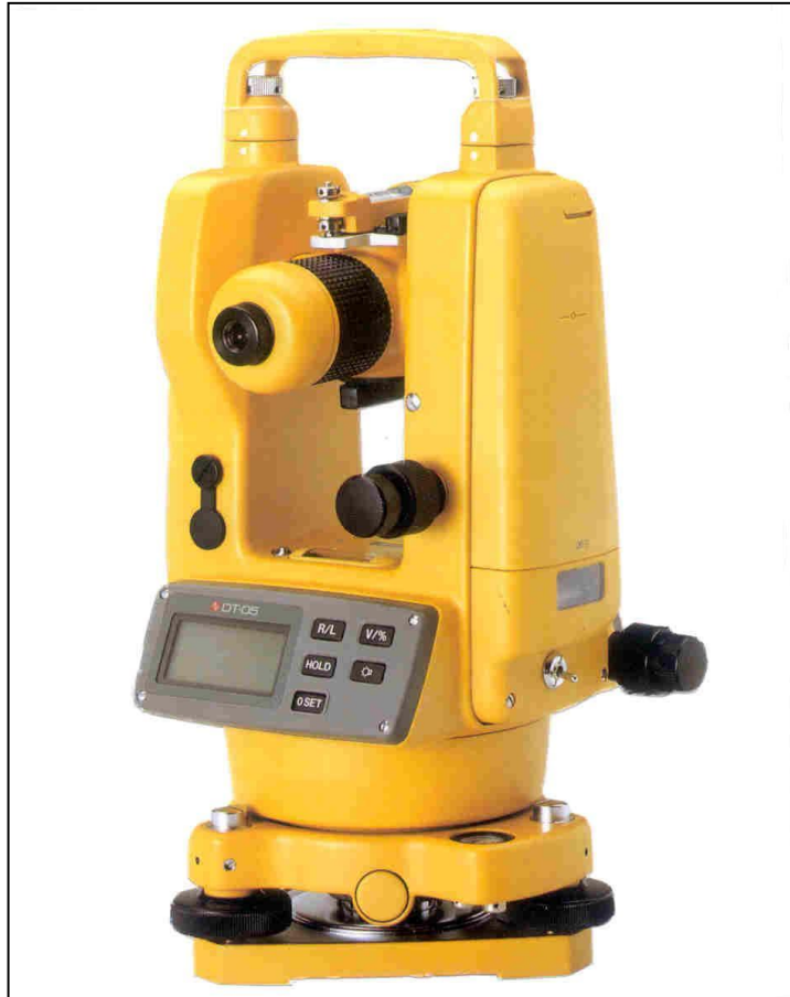
FIGURE 5.14: An example of a digital theodolite.
