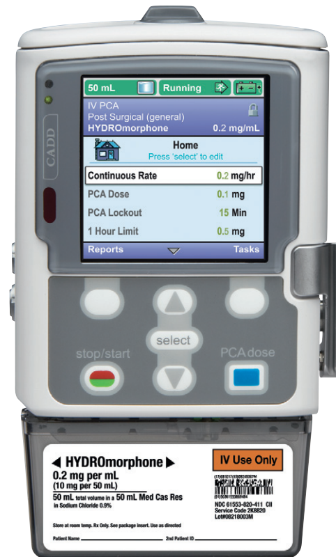
FIGURE 5-7 A patient-controlled analgesia infusion pump. (Courtesy Smiths Medical ASD, Inc., St. Paul, Minnesota.)
