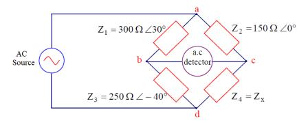
Given the AC bridge of the Figure in balance, find the components of the unknown arm  $Z_x$
