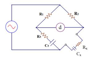
A similar angle bridge is used to measure a capacitive impedance at a frequency of 2 kHz. The bridge constants at balance are  $C_3=100~\mu\text{F},~R_1=10\text{k}~\Omega,~R_2=50~\text{k}~\Omega,~R_3=100~\text{k}~\Omega.$
