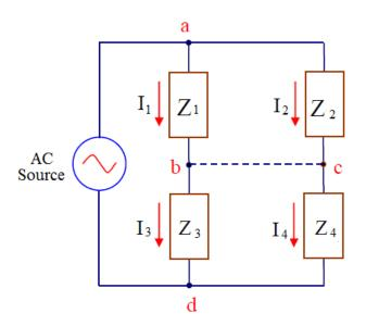
The impedance of the AC bridge are given as shown in the Figure. Determine the value of the unknown arm.
