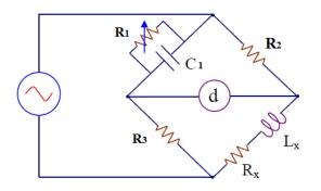
A Maxwell bridge is used to measure an inductive impedance. The bridge constants at balance are  $C_1=0.01~\mu\text{F},~R_1=470\text{k}~\Omega,~R_2=5.1~\text{k}~\Omega,~R_3=100~\text{k}~\Omega.$
