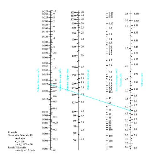
Specify the required size of Schedule 40 steel pipe to carry 0.034 m<sup>3</sup>/s of water with no more than 4.0 m of head loss over a 1000 m length of pipe. Use the design value for  $C_h$ .
