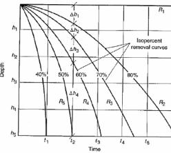
The advantage of the experiment is that it is possible to obtain removal data at various depths of settling.
