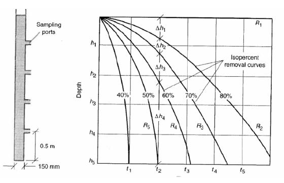
The total fraction of particles removed for a continuous distribution:
