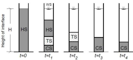
The corresponding interface settling curve
