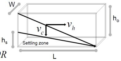
τ: residence time V=Wh<sub>o</sub>L: volume of tank A<sub>s</sub>: top surface area of tank
