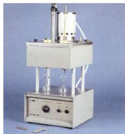
Saybolt Viscosity Test (Petroleum Products at Specified Temperatures between 70° and 210° F)
