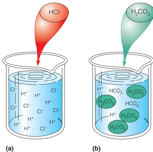
**FIGURE 15.11** Dissociation of strong and weak acids. **(a)** When HCl, a strong acid, is added to water it dissociates completely into its ions ( $\text{H}^+$  and  $\text{Cl}^-$ ). **(b)** By contrast, dissociation of  $\text{H}_2\text{CO}_3$ , a weak acid, is very incomplete, and some molecules of  $\text{H}_2\text{CO}_3$  remain undissociated (symbols shown in green ovals) in solution.
