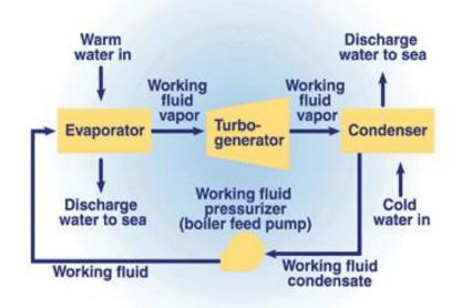
In the closed-cycle OTEC system, warm seawater vaporizes a working fluid, such as ammonia, flowing through a heat exchanger (evaporator). The vapor expands at moderate pressures and turns a turbine coupled to a generator that produces electricity. The vapor is then condensed in condenser using cold seawater pumped from the ocean's depths through a coldwater pipe.
