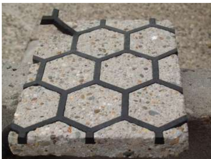
Plate 19 – Hexagonal rubber floor template
