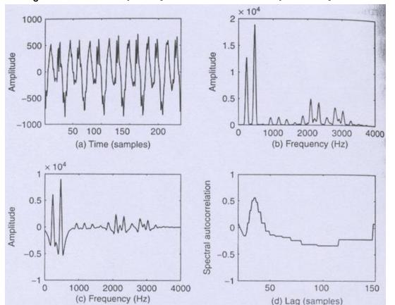
(a) Speech signal (8 kHz)(b) Magnitude spectrum(c) Zero-crossing spectrum(d) SA function
