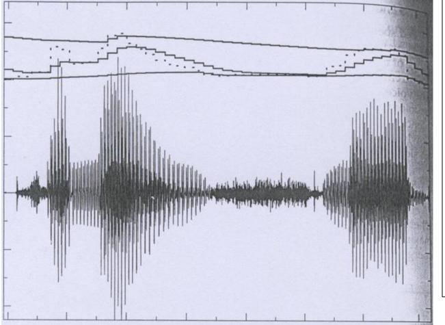
$E_{\max}(n)$  track  $E_{av}(n)$  track  $E_{\min}(n)$  track Dotted: frame energy Speech waveform Decision logic: If  $\{(E_0 > E_{max} - TH1) \text{ or }$  $(E_0 > E_{av})$ } Voiced, Else if  $(E_0 < E_{\min} + TH2)$ Unvoiced, Else Not-sure.
