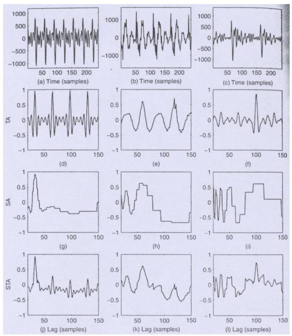
□ Analysis of the effect of the STA weighting factor  $\alpha$  in terms of the pitch error rate
