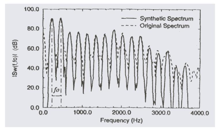
Pitch estimation using spectral autocorrelation
