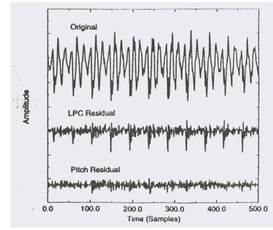
No longer the sharp pulse-like characteristics in pitch residual signal
