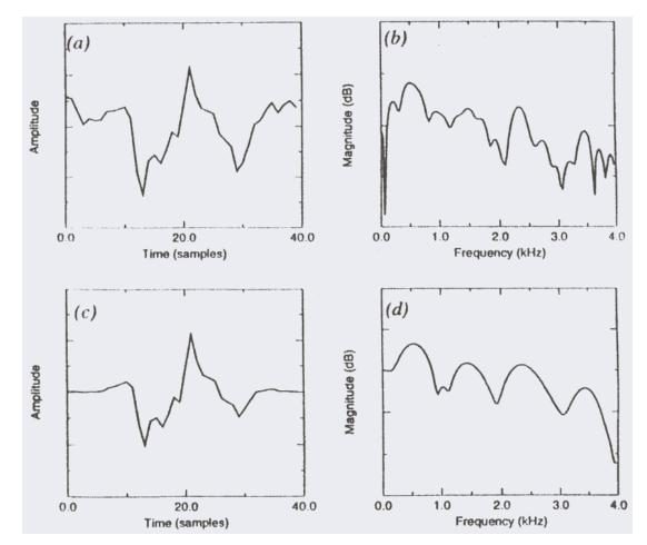
(a), (b): using rectangular(c), (d): using Hamming
