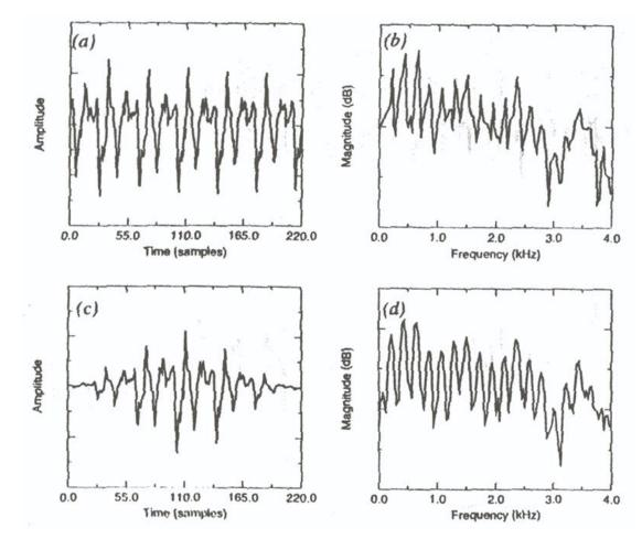
(a), (b): using rectangular(c), (d): using Hamming
