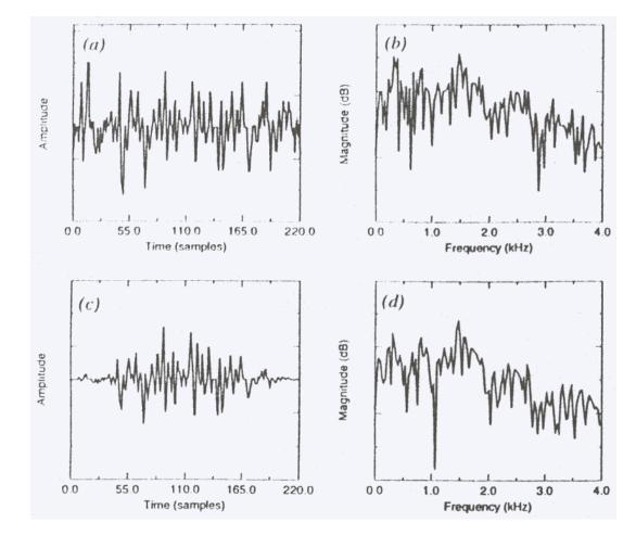
(a), (b): using rectangular(c), (d): using Hamming
